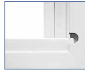
Tight mortise-cut, double-wall sill dam extends inside the jamb, eliminating the need to caulk an open seam.
