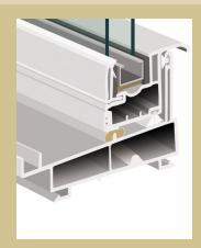
Soft-Seal<sup>TM</sup> straddle gasket is a closed-cell neoprene cushion-gasket under the sash that straddles the sill rail and helps prevent air and water infiltration.
